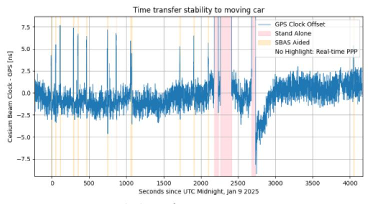
Even in high interference environments, L5 capable receivers hold robust solutions
