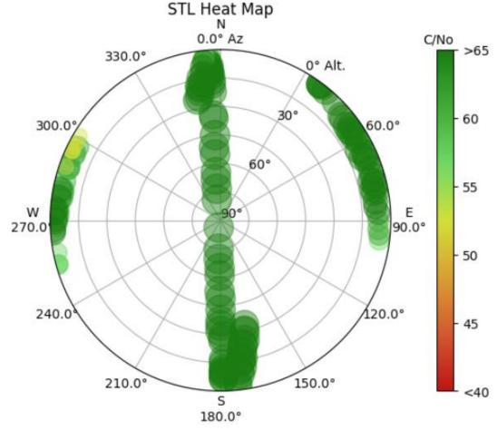
This plot shows the rapid movement of LEO (STL) satellites during a 12-minute period traversing the sky from horizon to horizon
