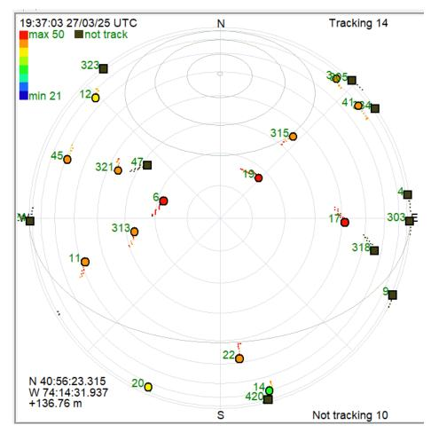
This plot shows the slow movement of GNSS satellites during a 12-minute period each moving only a few degrees
