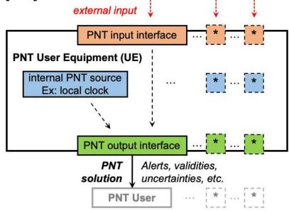
\* The generic PNT UE Model can encompass any number of input interfaces, internal PNT sources, output interfaces, and PNT users.
