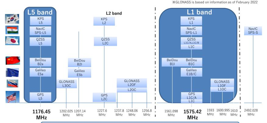
Multi-band GNSS receiver can receive multiple GNSS frequency bands
