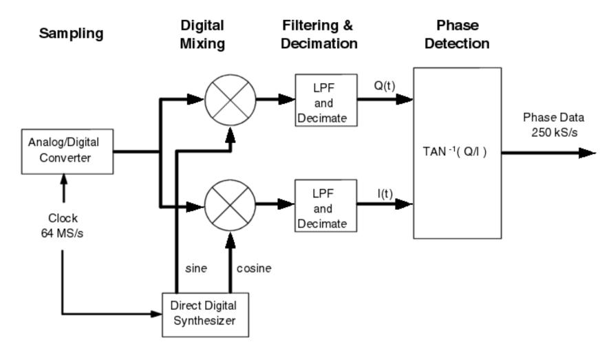
A local oscillator synthesized from the internal clock down-converts the input to base-band where the samples are used to compute the phase difference between the LO and the input.
