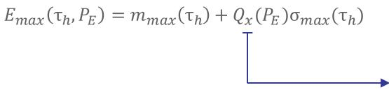
Q converts RMS to Peak for a specified error rate, P<sub>E</sub>
