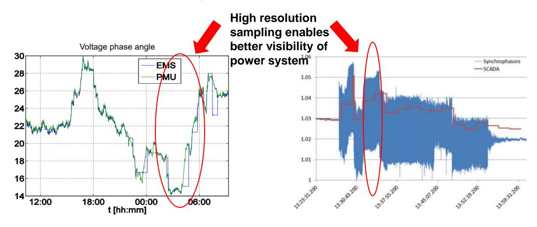
Conventionally timestamped SCADA measurements do not capture and analyze power system oscillations and disturbances sufficiently.
