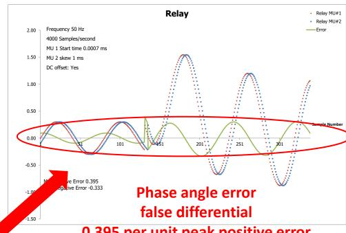
1 ms timing error leads to false operation
