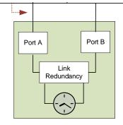
MU 1 receives PTP frames cascaded through IED 1 acting as boundary clock.
