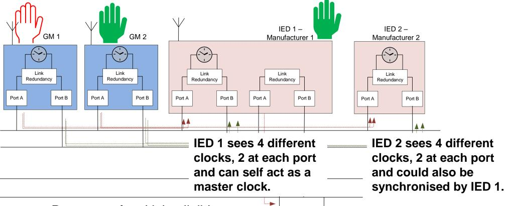
Presence of multiple eligible time sources and different implementations of BMCA by IED manufacturers can make the whole system unstable.
