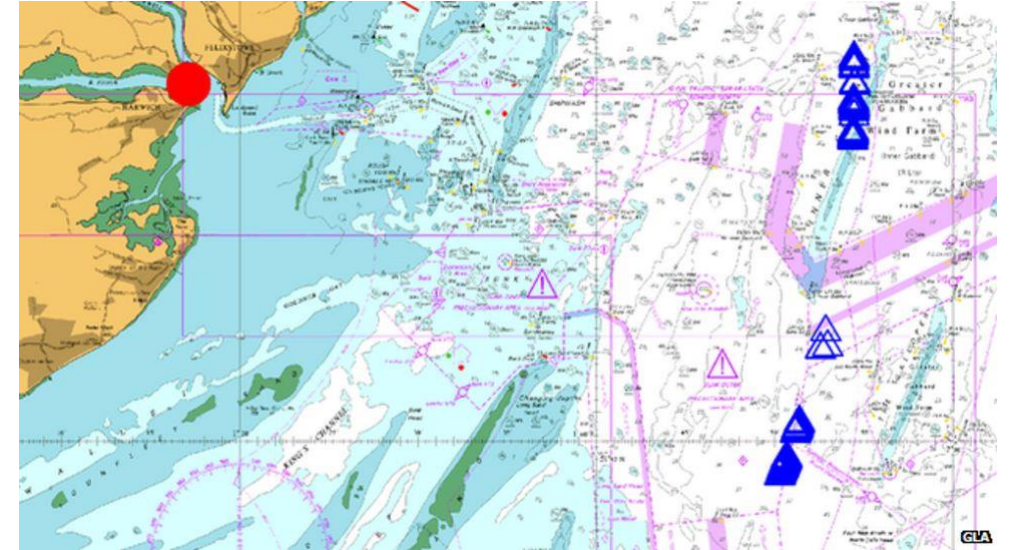
A UK GLONASS receiver with true position given by red dot, reports its position as being coincident with blue triangles on map - Image from BBC
