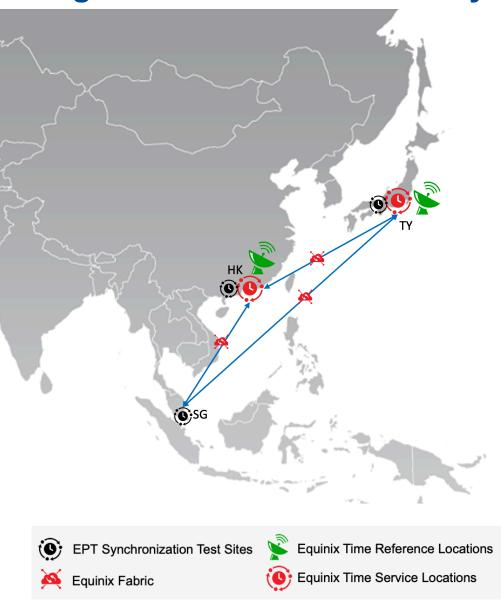
> Typical cross metro, PTP accuracy observed is ~1.5µs over Equinix Fabric
