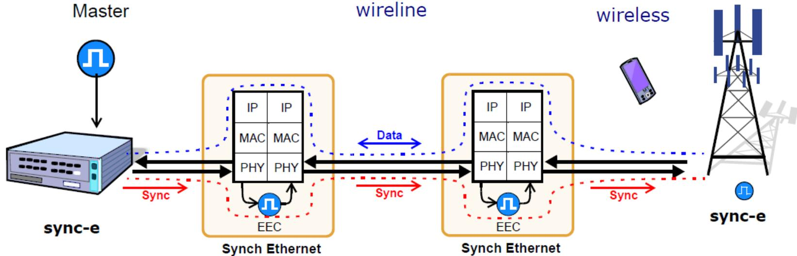
Also referred as **Sync-E**, is an ITU-T standard for computer networking that facilitates the transference of frequency reference signals over the [Ethernet physical layer](#). This signal can then be made traceable to an external clock.
