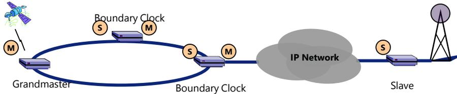
***A Boundary Clock has an internal oscillator and can extend the reach, and/or offload slave capacity from the PTP Grandmaster.***
