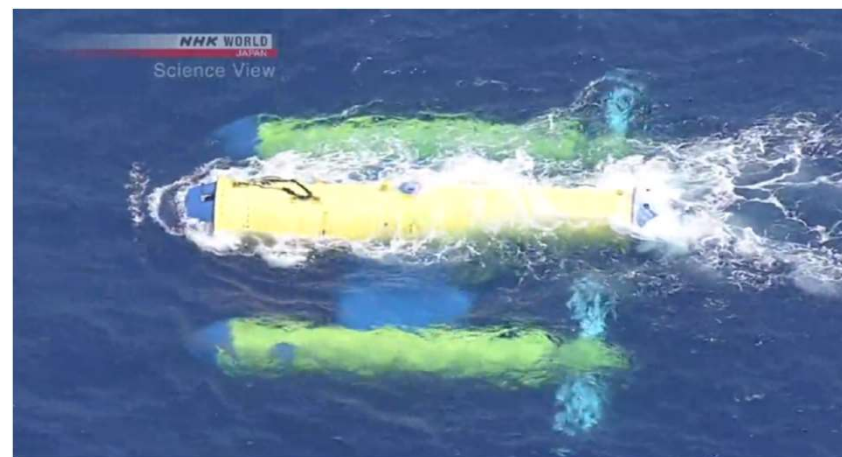
50kW Marine Generating Unit, Trial Operation 2017
