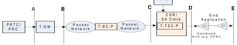
The PRTC is co-located with the Boundary Clock – Greenfield deployment of GPS in first cell aggregation node, or indoor cells
