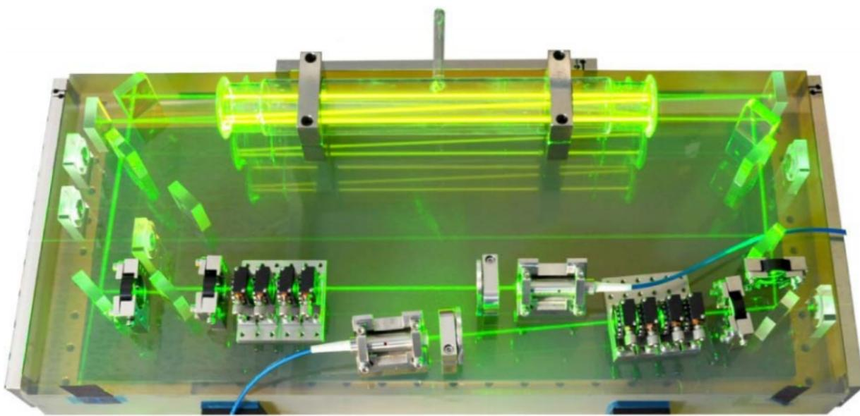
**Fig. 1.** Photograph of the integrated EBB setup. Optics are joined to a thermally and mechanically highly stable glass baseplate made from OHARA Clearceram-HS using adhesive bonding technology. The footprint of the EBB baseplate is 550 mm × 250 mm. The length of the iodine cell is 30 cm.
