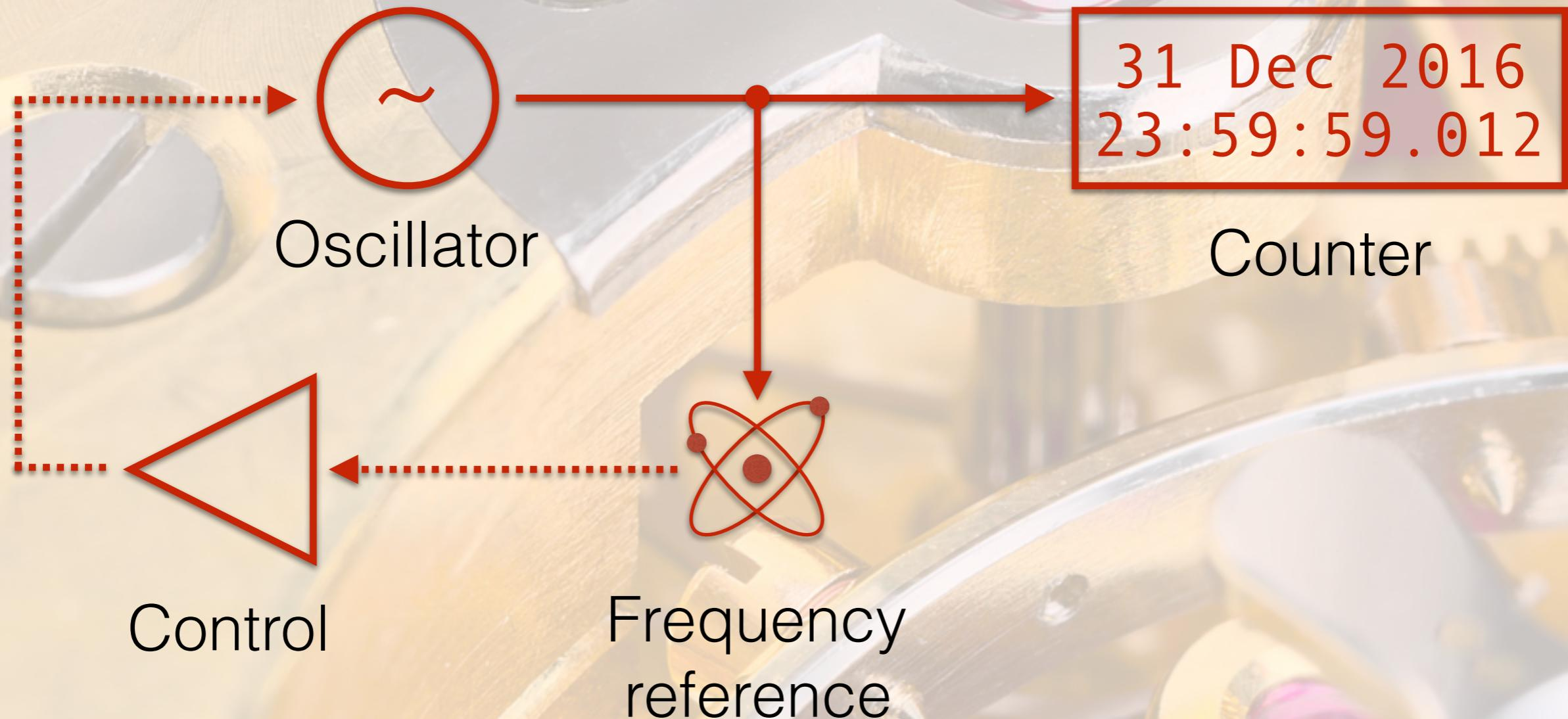
“Count cycles of an oscillator, which is itself referenced to a minimally-perturbed atomic resonance.”
