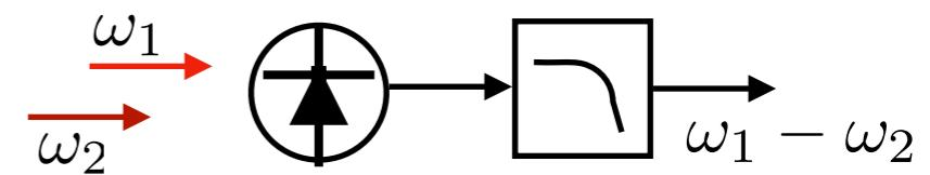
“Interference on a photodiode”
