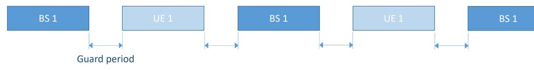
• If synchronization is poor between cells, a neighbouring cell transmission can interfere with UE transmissions:
