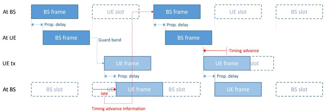
• Timing advance is a measure of round trip delay, and can be used to compensate BS sync
