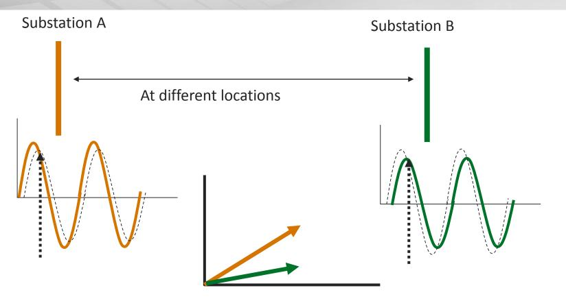
By synchronizing the sampling processes for different signals, which may be hundreds of miles apart, it is possible to put their phasors on the same phasor diagram.
