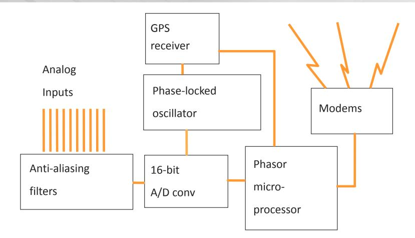
Except for synchronization, the hardware is the same as that of a digital fault recorder or a digital relay.
