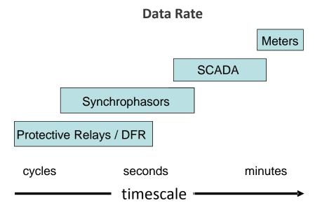
Time synchronized data can be gathered at sample rates much faster than traditional supervisory control and data acquisition (SCADA) systems, and provide the missing link between localized digital fault recorders (DFR) and SCADA systems, which are much slower. However, unlike most SCADA systems, these emerging wide-area measurement technologies utilize Internet protocols to exchange measurement information.
