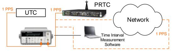
• "Packet" (Dual Point Measurement) Measurements are constructed from packets time-stamped at two points – in general two pieces of equipment, each with a reference, at two different locations – are needed
